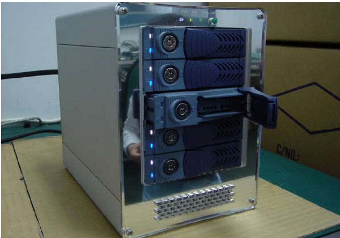
Array manager – HDD3 lost and rebuild to HDD5 ( Spare HDD ) and Burning program still keep running
